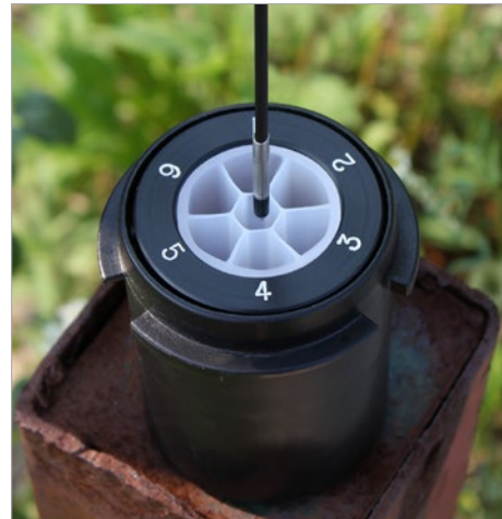
Measure Water Levels within the narrow channels of a Solinst CMT® System.
